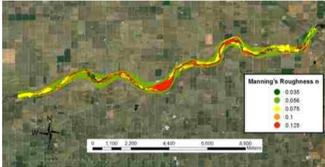
Figure 4: Reach 1B overview of default Manning's n values as provided by Reclamation (2012)
